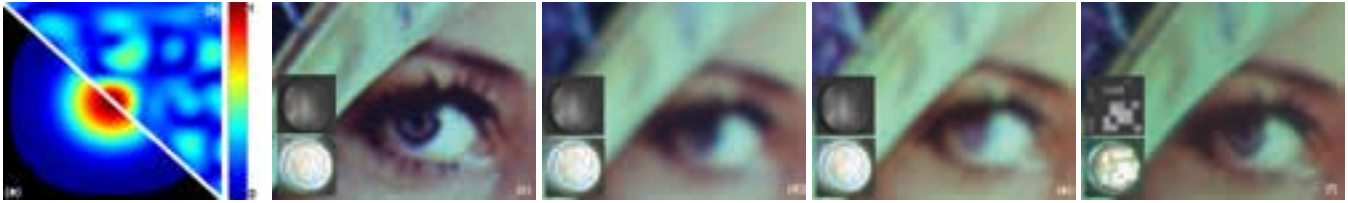
Figure 1: The power spectra of a Gaussian PSF (a) and of the PSF of a coded aperture (b): Fourier magnitudes that are too low are clipped (black), which causes ringing artifacts. Image projected in focus (c), and with the same optical defocus (approx. 2m distance to focal plane) in three different ways: with spherical aperture – untreated (d) and deconvolved with Gaussian PSF (e), with coded aperture and deconvolved with PSF of aperture code (f). The sub-images in c-f are photographs of the apertures and their captured PSFs.
