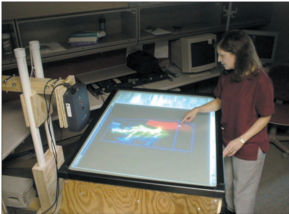
Figure 1: The SMARTBoard is mounted horizontally on a frame.
