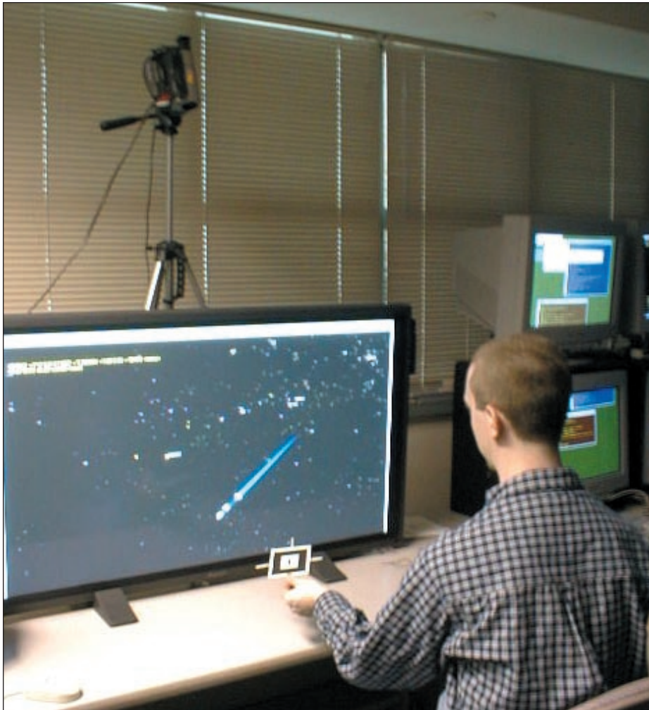
Figure 2: The Virtual Director application, with camera mounted atop a plasma panel.
