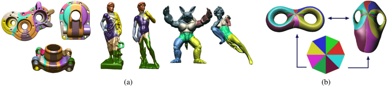
Figure 9: Solving cross-surface mapping for high-genus surfaces. (a) Mapping by divide-and-conquer through consistent surface decomposition [Li et al. 2009a], (b) global optimization on the covering space with uniformization metrics [Li et al. 2008].
