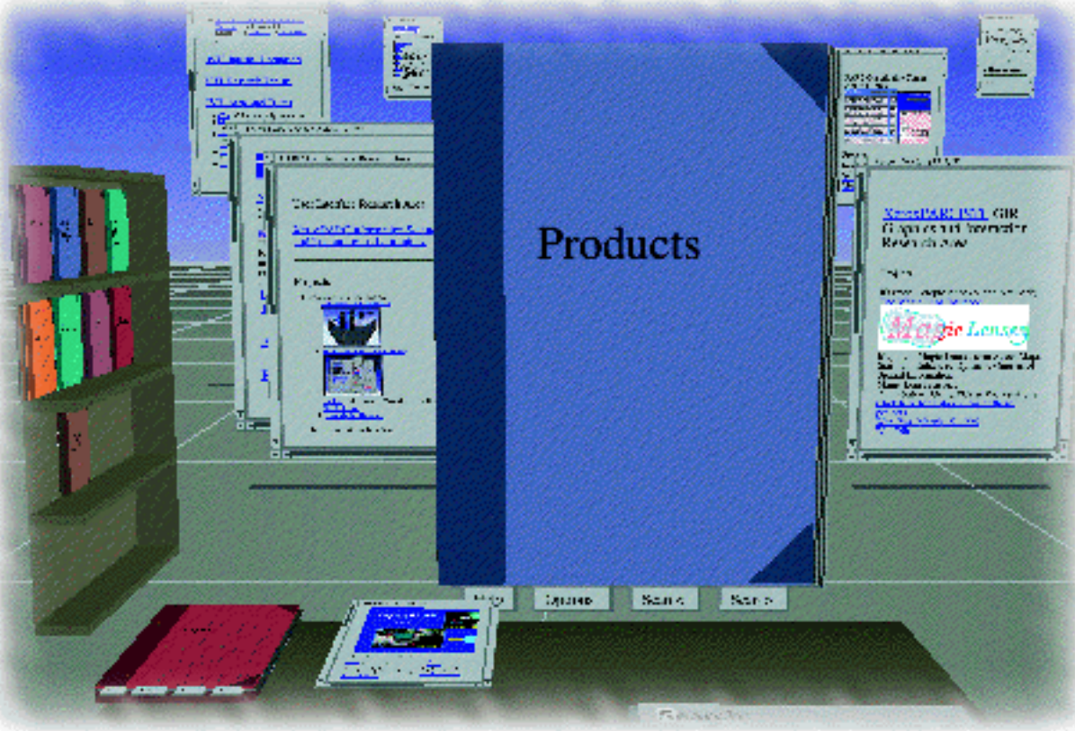
Figure 3. The Workspace metaphor developed at Xerox PARC is used to organize WWW information [Robertson, et al, 1996].
